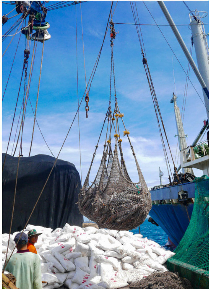
Photo 1: Transshipment Sling Structure
