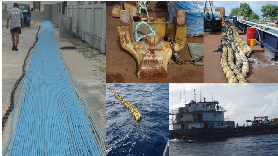
FAD materials and deployment
